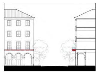
The façade should clearly express the distinction between the ground level and the upper floors of a building to create a clear base.
