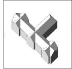
Simple roof and building forms like the ones shown here are encouraged. The predominant roof plan should be a rectangle or a combination of rectangles. Building massing should be composed of simple, rational forms. Roof forms should be pitched, gabled, or hipped. Flat roofs should only be used for parking garages.
