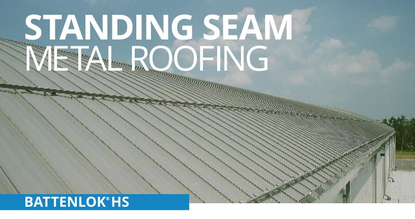
BattenLok® HS is a mechanically field seamed, high strength structural standing seam roof system. The BattenLok® HS panels have a 2" tall vertical seam and are available in both 12-inch and 16-inch widths. BattenLok® HS can be installed directly over purlins or bar joists and is capable of transitioning from roof to fascia. BattenLok® HS does not require a solid substructure for support.
