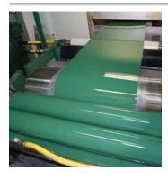
Berridge owns and operates its own continuous coil-coating paint line to provide fast, responsive service for coil and flat sheets. A wide array of long-life Kynar 500° /Hylar 5000° Berridge colors are available pre-slit for portable roll forming or in flat sheet form for custom trim and flashing fabrication. Branch locations have a large inventory of 24 gauge painted flat sheets in all our standard colors and slit coil in popular widths and colors for immediate pick up.
