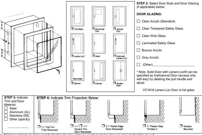
Trimless cabinets must be installed before the drywall because their plaster stops must be behind the drywall. Trimless cabinets are not recommended for block wall installation.
