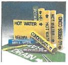
MS-970 coiled plastic pipe markers are designed to identify piping in a wide variety of environments. They stay in place on pipes due to the memory of the coiling process and therefore do not rely on a pressure-sensitive adhesive. No preparation of the pipe surface is required for application, so installation time is reduced compared to conventional stick-on marker systems. Legends are sub-surface printed so they are protected by a layer of plastic.
