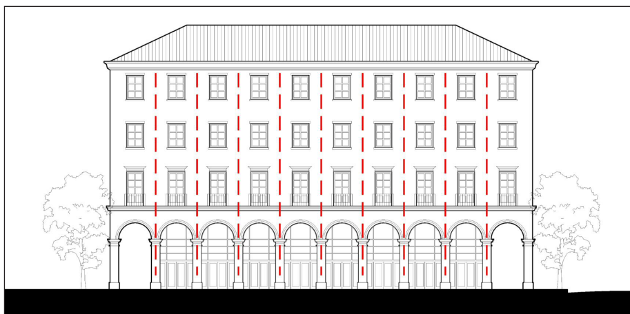
To avoid a monolithic appearance, façades shall be vertically articulated with bays no larger than 25 feet in width.
