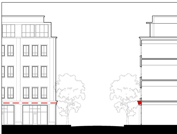
Buildings shall be articulated to break down the scale into a tri-partite vertical organization (base, middle, and top).
