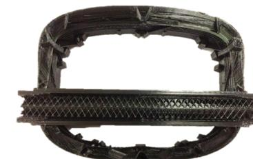
Figure 12. Failed Stiffener Test
