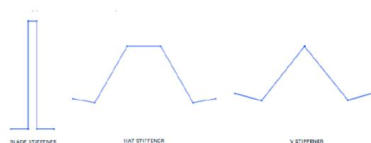
Figure 3. Stiffener Cross-Sections
