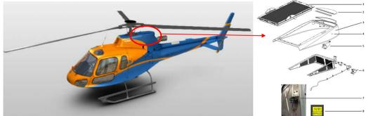
Figure 1. AS350 B3/H125 Helicopter and IBF System
