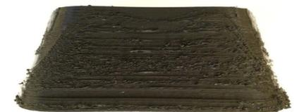
Figure 13. Bulging Material Failure
