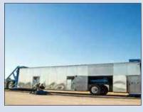
moves back and forth over a test section every six seconds to simulate stress and measure durability of various materials used to pave roads.
