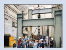
and conventional materials can be tested, and the laboratory is capable of simulating the effects of earthquake, blast and wind forces on the performance of structures.
