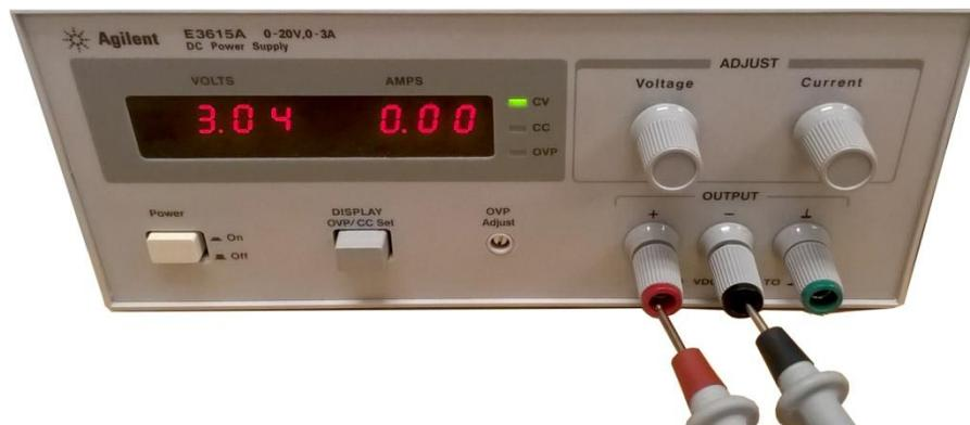
Figure 4: Directly measure the DC voltage from the power supply.
