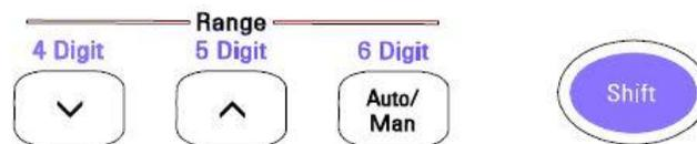
Figure 6: Pressing Shift will allow you to access the blue alternate keys.
