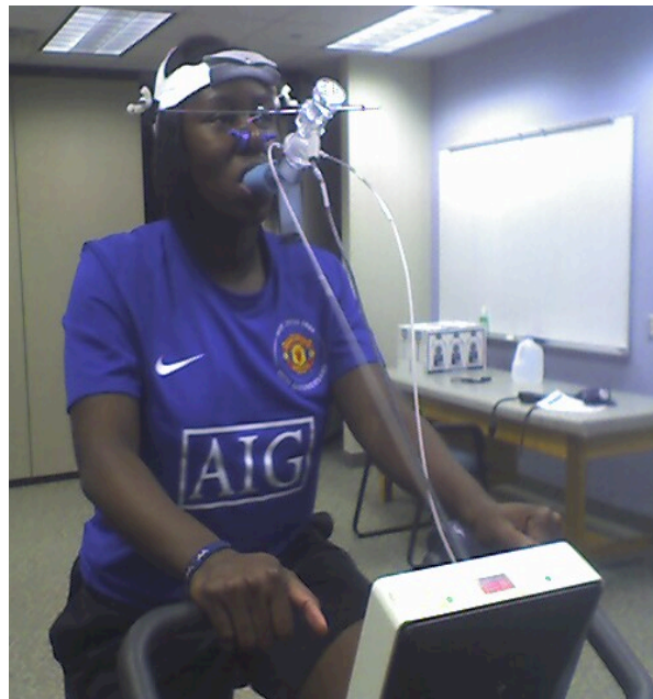
Diagram 2.6: A Subject on top of the Cycle Ergometer Strapped to the Sensormedics Metabolic Cart
