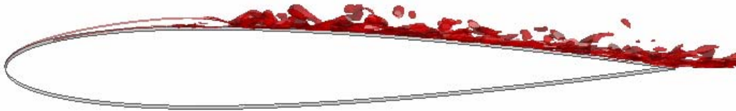
Fig. 10. Isosurface of instantaneous spanwise vorticity ( \omega_y = 30 )
