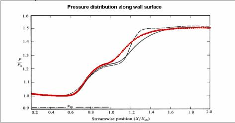
Figure 3.8 Comparison of pressure distribution on the wall surface. (The red one is our computation, the black dash one and solid one are Degrez's computation and experiment respectively)
