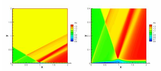
Figure 3.5 Density distribution: left is a normal view and right is stretched in the normal direction by a factor of 5
