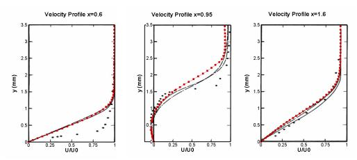
Figure 3.9 Comparison of velocity profiles at different locations (The red one is our computation, the black solid line and black square are Degrez's computation and experiment respectively)
