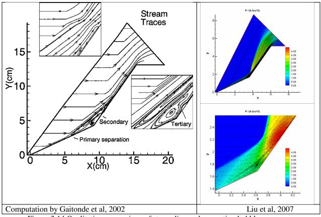
Figure 3.14 Qualitative comparison of streamline and separation bubble
