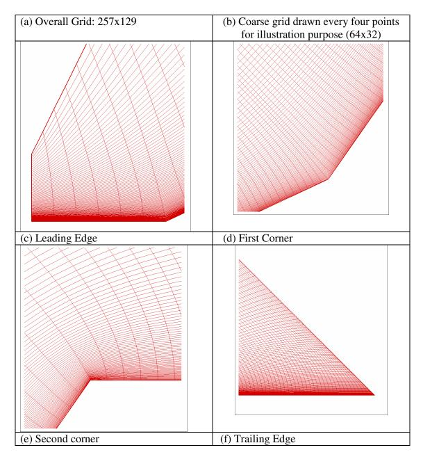
Figure 3.11. Elliptic Grid Generation
