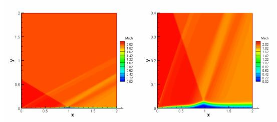
Figure 3.6 Mach number distribution: left is a normal view and right is stretched in the normal direction by a factor of 5
