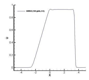
Figure 2.3 WENO for 1-D shock tube (T=2, grid=100)
