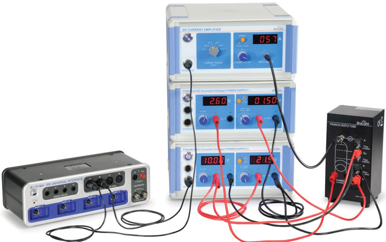
Figure 3: Frank-Hertz experimental setup
